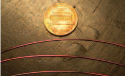
Figure 11. Optoelectronic fibre produced by MIT
