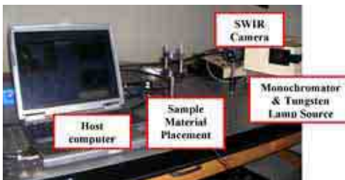
Figure 12. Optical bench with experimental apparatus
