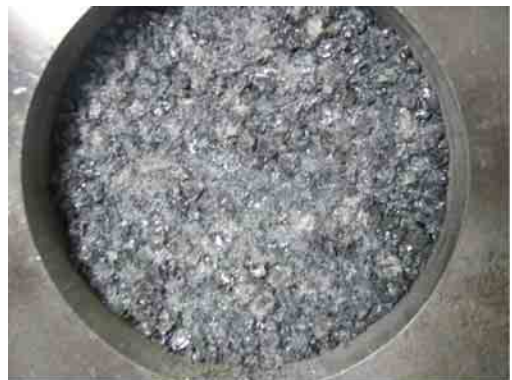
Figure 9: 305mm SiC compressed to 440MPa
