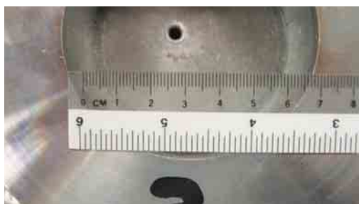
Figure 11. Projectile impact on 3-5mm SiC test specimen
