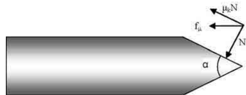
Figure 7: Frictional forces acting on penetrator
