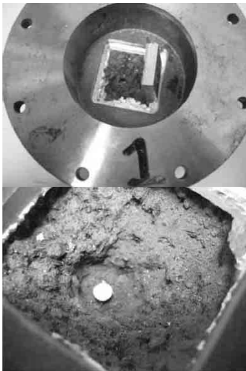
Figure 12. Projectile embedded in SiC test specimen 3-5
