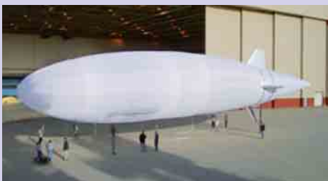
The Sanswire Stratellite™ is a specialized rigid airship that will operate in the stratosphere at 65,000 feet and be used to transmit various types of wireless communications by GlobeTel Communications in the USA. ( http://www.sanswire.com/ )
