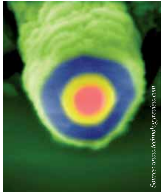
Cross-section of a nano-wire solar cell; just 300 nanometres wide, it could be used to provide organic steady power source at the microscopic level.
