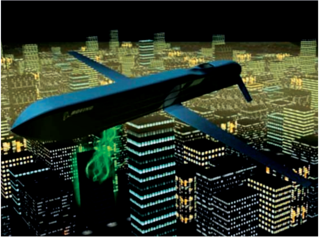
Figure 5: Boeing's Counter-Electronics High-Powered Microwave Missile (CHAMP) destroys electronic targets, not people. 12
