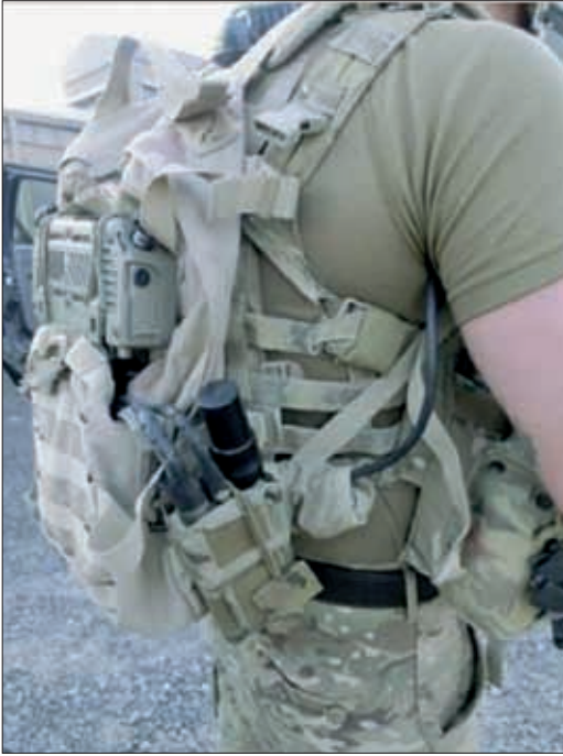
Illustration 3: A USAF Joint Terminal Attack Controller equipped with a Modular Tactical System (MTS), which includes a Tactical Mission Computer (TMC) that runs PSS-SOF mensuration software.
