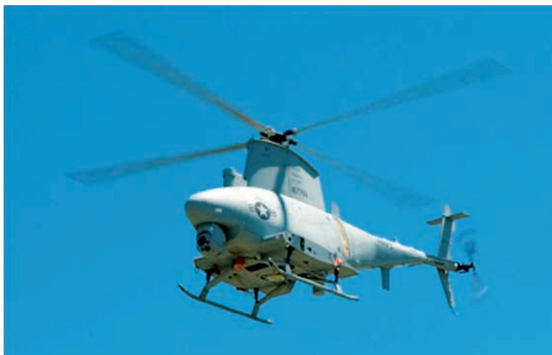
Figure 7: The US Navy's MQ-8 Fire Scout UAV can be equipped with the Tactical Synthetic Aperture Radar (TSAR), allowing it to see through dense foliage, clouds, and even sand or soil. 17
