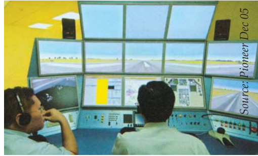
F-16C/D OFT capable of simulating emergencies, weather conditions and setting up 500 different scenarios
