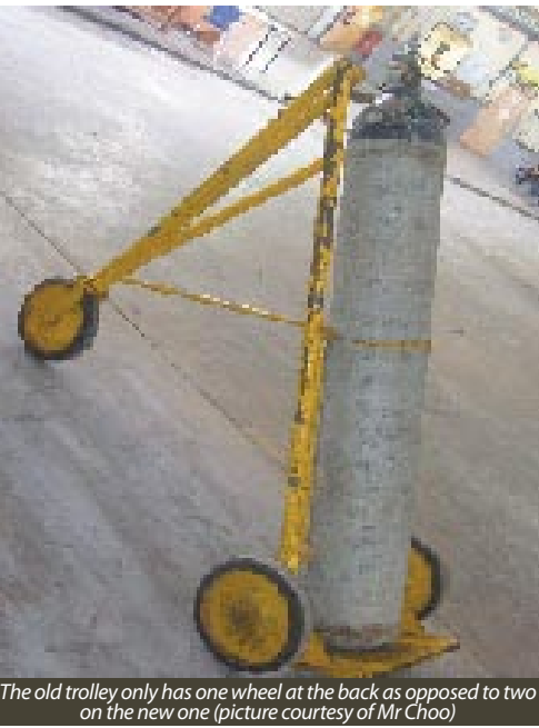
The old trolley only has one wheel at the back as opposed to two on the new one (picture courtesy of Mr Choo)
