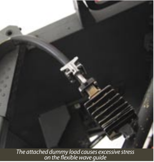
The attached dummy load causes excessive stress on the flexible wave guide
