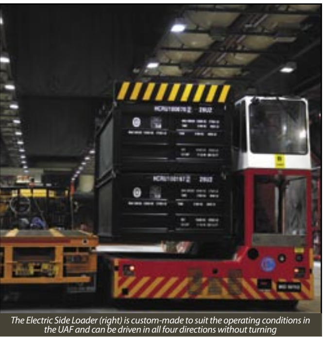
The Electric Side Loader (right) is custom-made to suit the operating conditions in the UAF and can be driven in all four directions without turning
