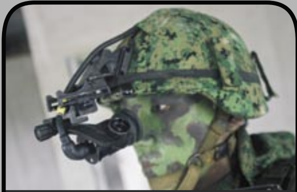
HEAD-MOUNTED DISPLAY. This displays digital maps and satellite images of the terrain, buildings and even locations of friendly and enemy troops to provide the commander with better situational awareness. The transparent display panel allows the user to maintain vision of his surrounding.
