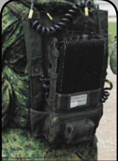
PORTABLE COMPUTER. The brain of the system. The current prototype weighs about 3kg, but future versions will be lighter.
