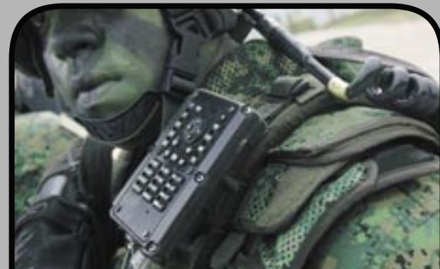
COMMUNICATION KEYPAD. This allows soldiers to send text messages, SMS-style, while still keeping an eye out for the enemy. It has hotkeys like 'On-Contact' and 'Call-for-Medic' which facilitate requests for assistance at the push of a button.
