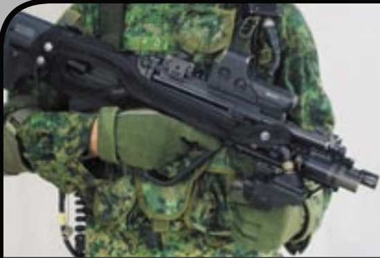
Section Commanders will also be equipped with a camera mounted on a special SAR 21 rifle. It takes snapshots of targets, which can be sent to friendly units to request for support fire. It also allows the Section Commander to aim the weapon around a corner without exposing himself to danger.
