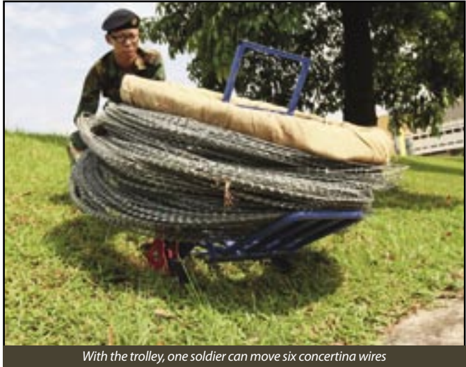
With the trolley, one soldier can move six concertina wires
