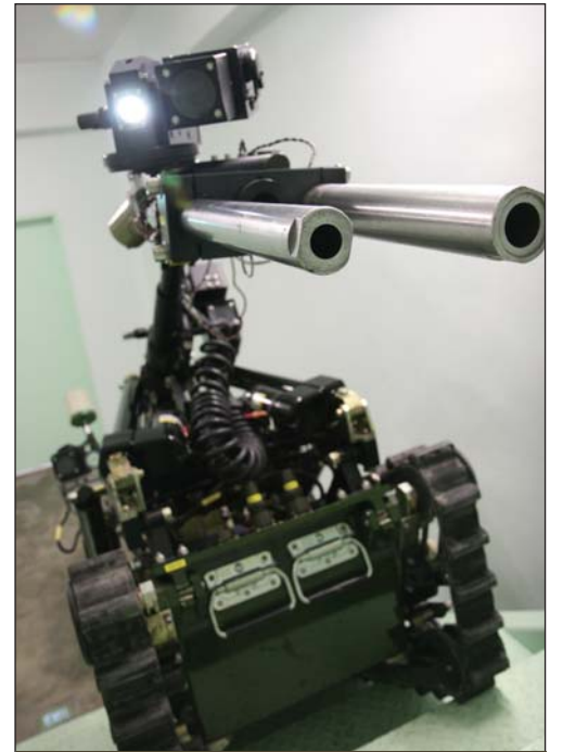
The Wheelbarrow Mark VIII robot can navigate obstacles and staircases to locate and neutralise CBRE threats. It can be remotely controlled to provide visual feedback on a situation, or destroy an IED.
