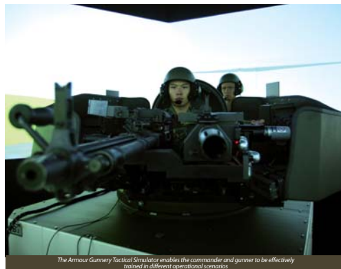
The Armour Gunnery Tactical Simulator enables the commander and gunner to be effectively trained in different operational scenarios.
