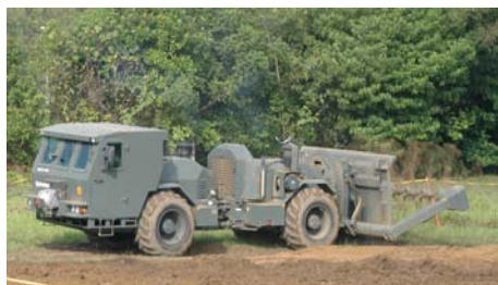
The Mine Clearing Vehicle is equipped with a motorised flail that whips the ground at high speed, destroying or detonating any mine embedded in the soil
