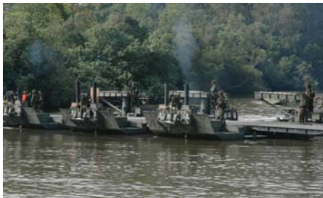
The COMET can join up to form a large raft capable of transporting even tanks and five tonners across rivers with ease
