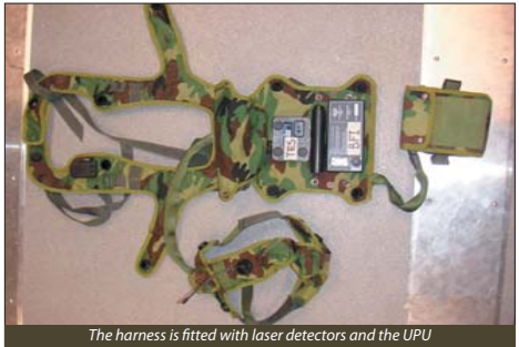
The harness is fitted with laser detectors and the UPU
