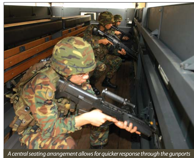
A central seating arrangement allows for quicker response through the gunports
