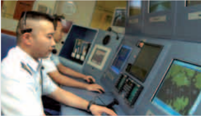
The Instructor Operator Station of the F-55 OFT is located in the control room and managed by an instructor who will control and monitor the simulation training
