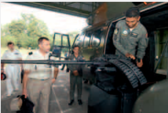
SSG Rajesh Saraj showing General Officer, International Affairs, FAF, BG Jean Albert Epitalon the features of a 0.5" calibre Heavy Machine Gun installed on a Super Puma helicopter.
