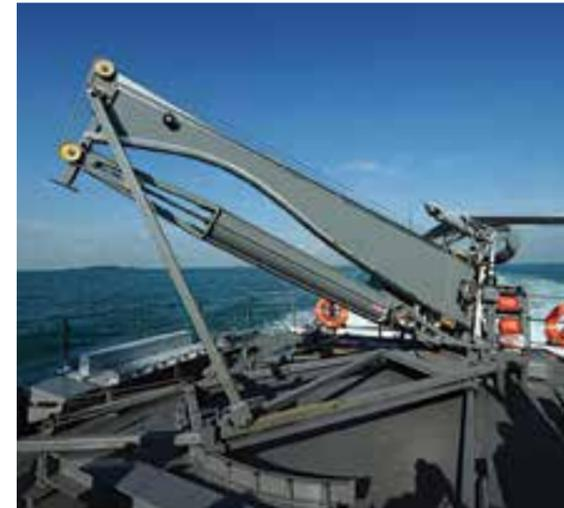
The design of the modified UAV launcher installed aboard the corvettes after the upgrade added additional functionality through a turntable.
