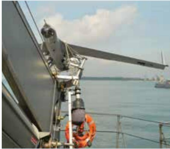
The ScanEagle UAV system was acquired as part of the missile corvette's upgrade programme to give it an organic surveillance capability. The ScanEagle UAV is made up of four components: the Launcher, the UAV, the Skyhook, and the Control Station.
