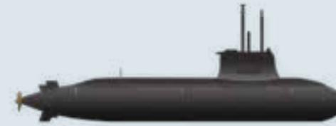
The Challenger-class submarines were purchased from Sweden in the 1990s. Their excellent hydrodynamic properties are achieved by its teardrop shape. This minimises hull resistance when the submarine is submerged. These submarines now form the Challenger-class submarine squadron of the RSN.
