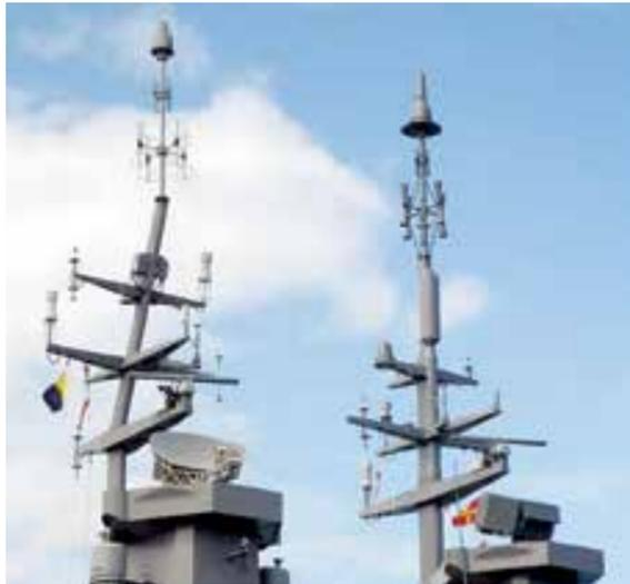
The pre-upgrade MCV with its slanted mast (left) compared to the upgraded MCV with its straight mast (right).
