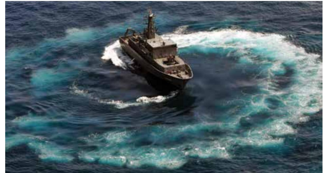
An MCMV demonstrating the sort of maneuverability provided by its Voith-Schneider propellers.
