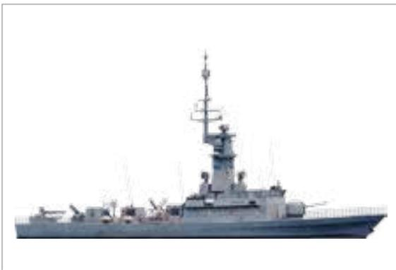
The post-upgrade MCV, with the straight mast configuration.
