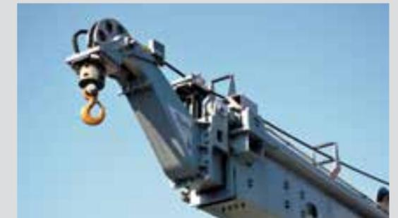
In addition, the team equipped the LARS with both automated and manual operations, making it easier for operators to manoeuvre through the small footprint of the SSM deck. With the automated operation, reliance on the crew's skills and judgement is reduced. This innovation has enhanced the safety and precision of operators without compromising the stealth and capability of the frigate.
