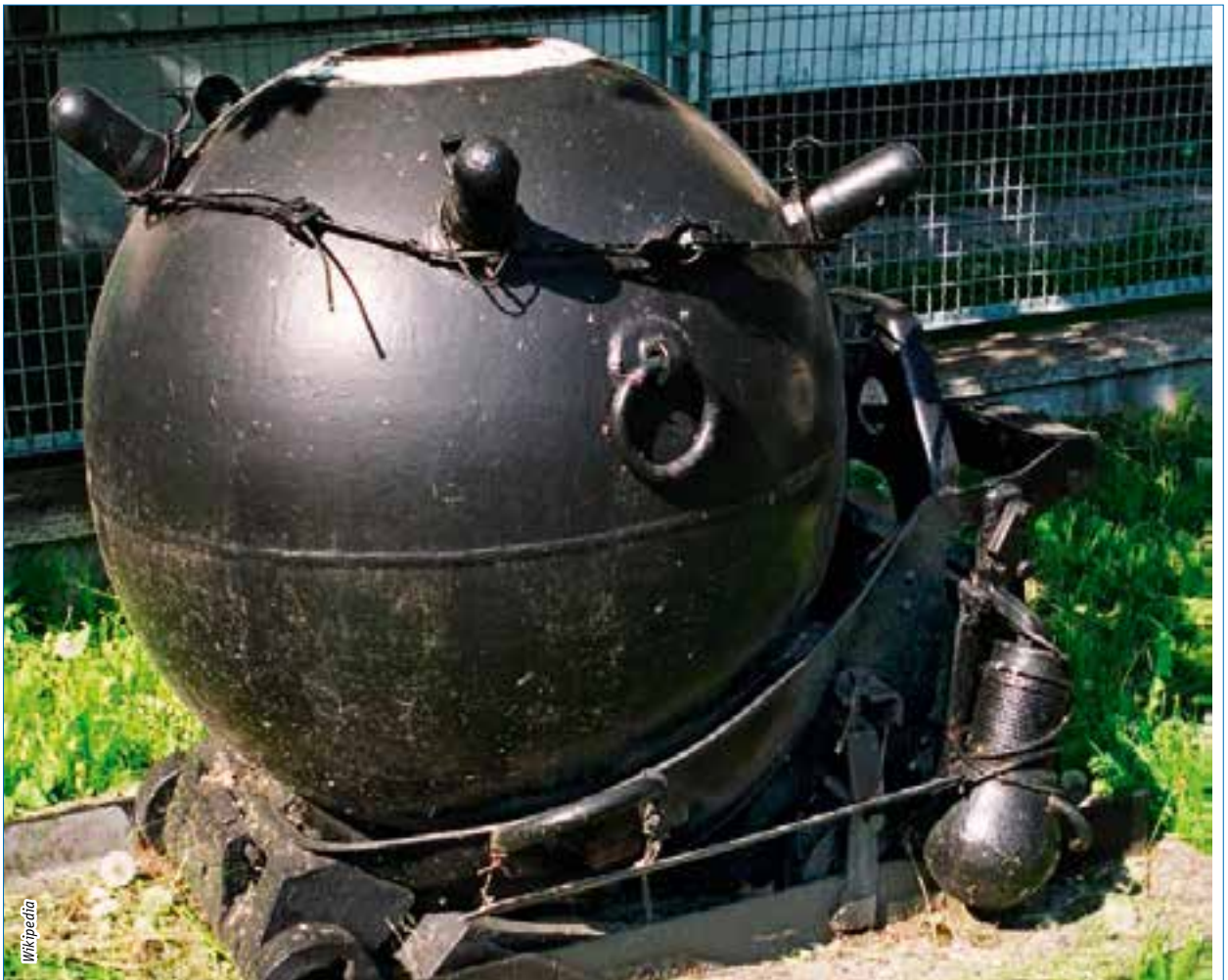
A Polish contact mine. When deployed, the protuberances near the top of the mine will trigger the mine's detonation upon contact with any ships out at sea.
