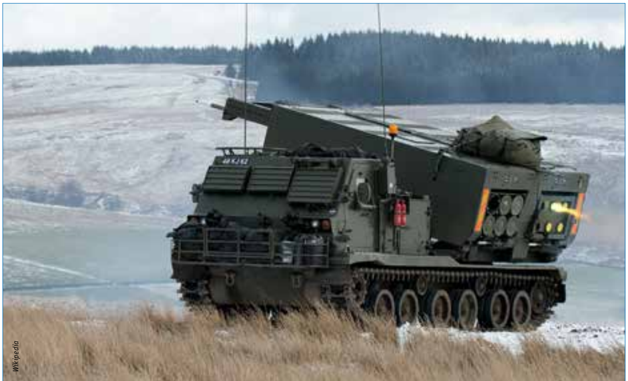
The British M270 Multiple Launch Rocket System (MLRS) firing a rocket during an exercise. The M270 is the original version of the MLRS, which features a weapon load of 12 rockets in two six-pack launch pod containers.
