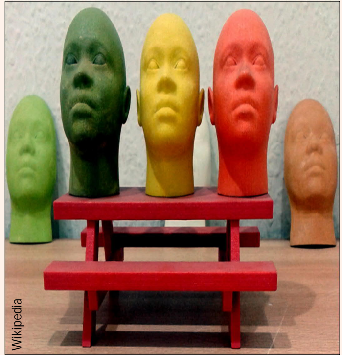
Miniature face models (from FaceGen) produced using Ceramic Based material on a Full Colour 3D Inkjet Printer .
