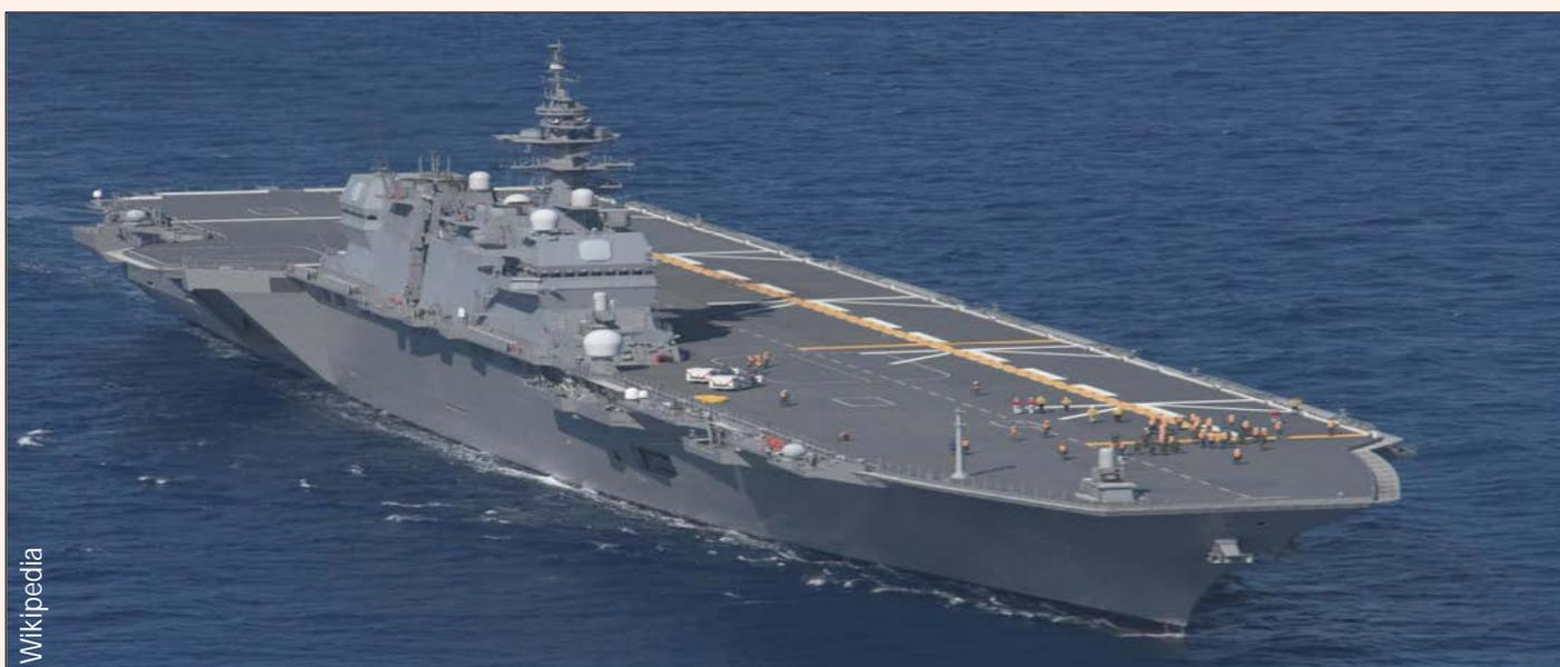
JS *Izumo* (DDH-183) with new markings and heat resistance coating on the flight deck, 3<sup>rd</sup> October 2021.
